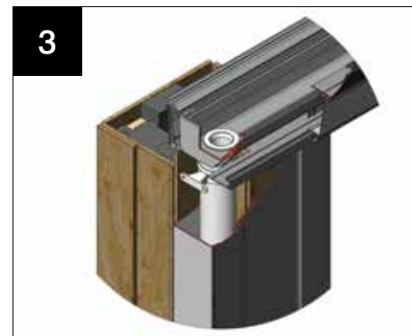
Cornice shown in situ with concealed downpipe.
