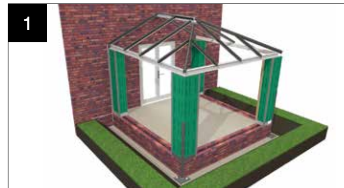
1 Fit eaves beam to columns. Fit roof skeleton.
