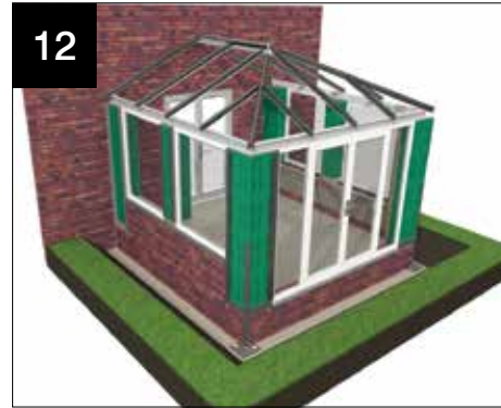
12 Fit and seal windows/doors against clips
