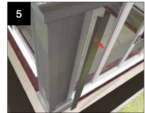
5 Clip on cladding as shown by locating inside clip first and rocking round the external clip. Repeat figs 4 and 5 to other side of the column.
