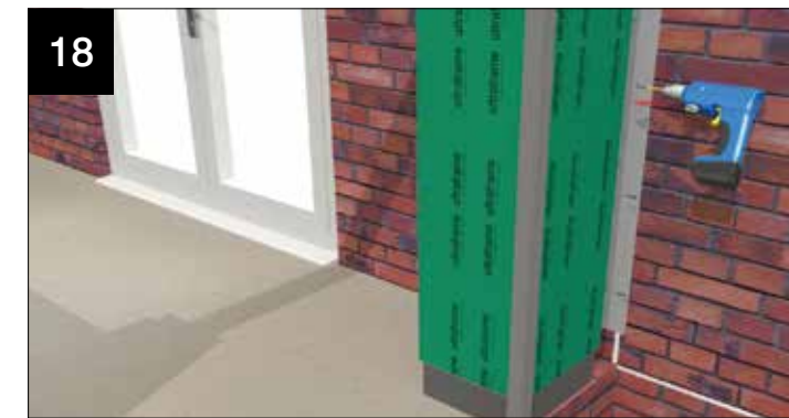
18 If an abutment is specified, permanently fix the column to the wall bracket using the screws supplied as shown (4.8 x 25mm pozi pan head self tap screw).
