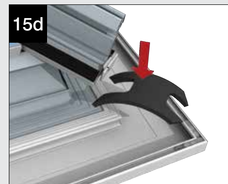
At 90° corner insert 'H' section and press down. Similarly apply at stop end or outlet positions.
