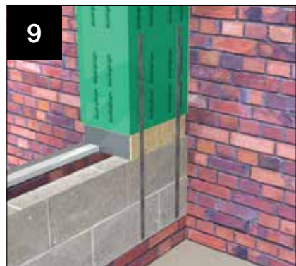
9 ABUTMENT Fasten straps down inside of wall of abutment column.
