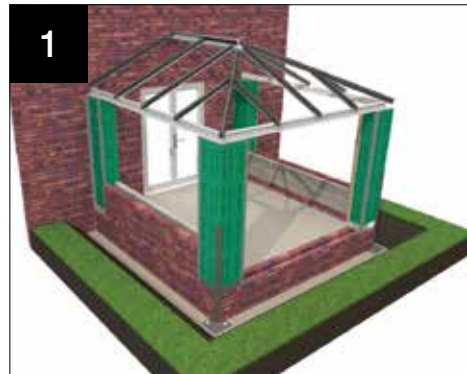
Fit windows between columns.
