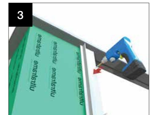
Push and hold the cladding clips in position and screw fix through the holes into the column both front and side using the 4.8 x 25mm pozi pan screws provided. SILICONE SEAL AGAINST THE CRN/1 OR CILL
